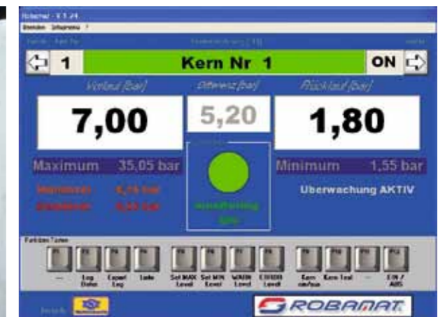
Visualization of core break monitoring, pressure sensors for measuring pressure differences
