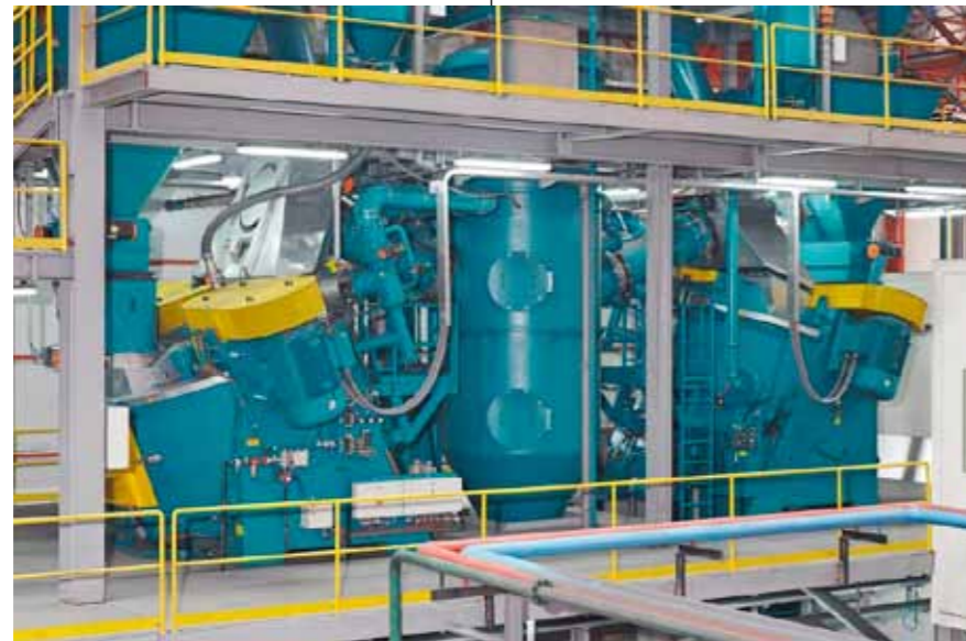
Twin system with two EIRICH Intensive Mixers type RV32VAC
