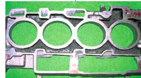
Figure 6: Veining and retained particulate levels prior to use of RHEOTEC XL coatings
