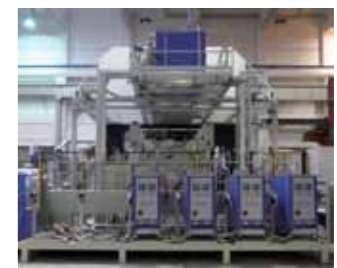
Die cooling with Robamat temperature control units
