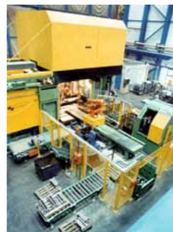
Fully automated GDK 2500 with optimized automation design
