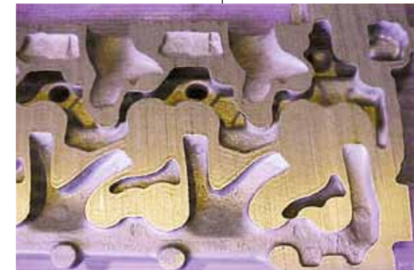
Figure 5: Defect free internal channels when using a single coating application of RHEOTEC XL
