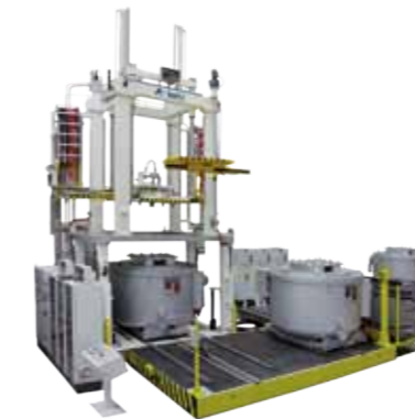
Low-pressure casting machine with furnace shuttle system
