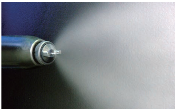
Lubrolene WFR-EC is applied by electrostatic spray.
