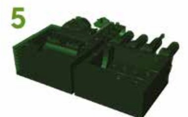
5 Removing the unbound sand. Sand mold or core is ready for casting.
