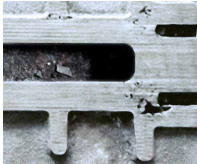
Casting results before and after the modified alloy additions 改变孕育合金前后的铸件
