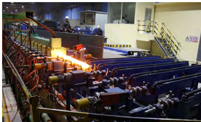
方坯感应加热 Induction heating of square billets
