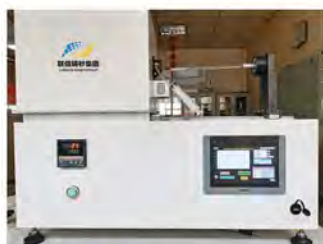
型砂发气量检测仪 Molding sand gas emission tester
