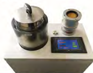
型砂透气性检测仪 Product-Molding sand permeability tester
