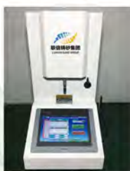
型砂抗折强度检测仪 Molding sand flexural strength tester
