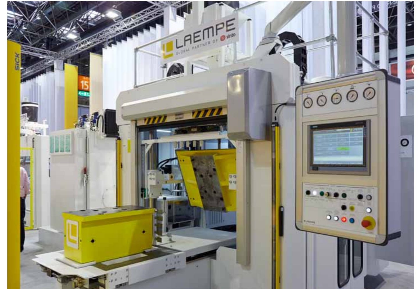
Keeping it accurate: LFB-series automatic core shooters offers high product quality for 24-hour continuous operation - thanks to the 4-post table guide the best possible precision can be achieved.
