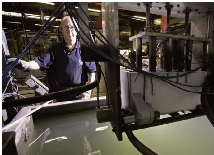
Image 3: As part of the leak test, the cast parts are tested for possible gas defects and porosities caused by shrinkage. In the area of boiler production in particular, the rejection rate due to gas defects was reduced by more than 5 % with ECOCURE SL.
