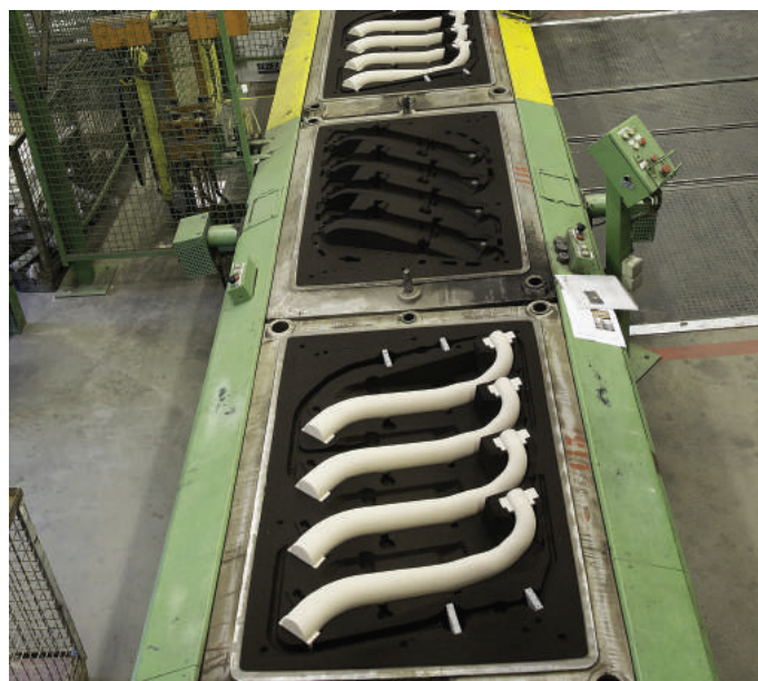
Image 8: MGG also uses a low-pressure sandcasting process that can be used to cast particularly thin-walled parts.
