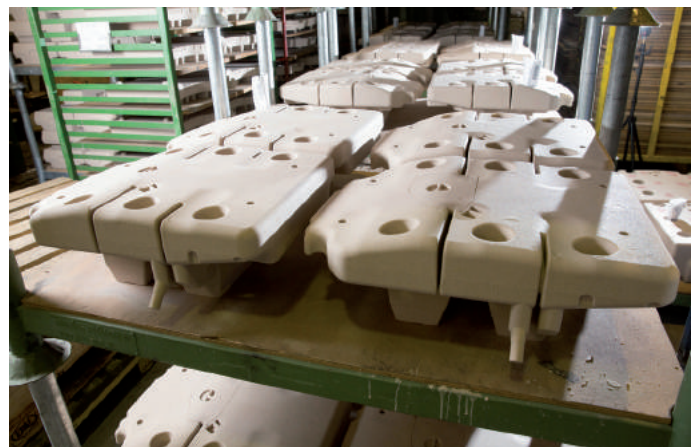
Image 6: The quantity of part 2 that needs to be added can be reduced by more than 20 % with the new ECOCURE SL system. Dosing quantities of the rival product: 0.52 % of part 1 and 0.52 % of part 2; dosing quantities of the ECOCURE SL system: 0.53 % of part 1 and 0.40 % of part 2.
