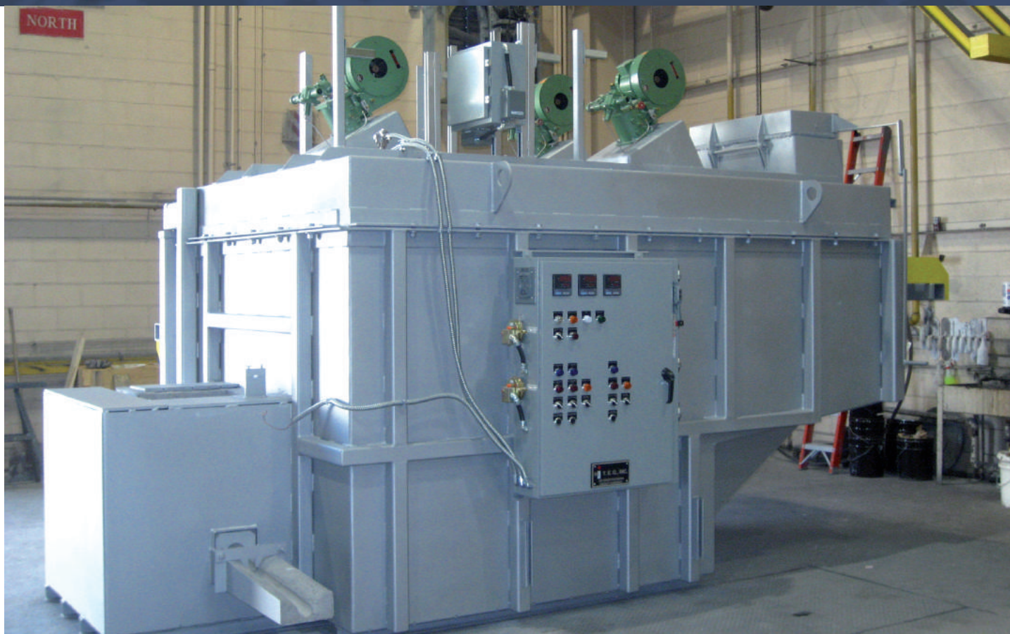
The HiTEQ™ "MiniMelter", 200 kg/h to 500 kg/h melt rate; Compact dual-chamber design - melting and holding directly at the casting station - eliminating molten metal transfer costs and temperature fluctuations.
