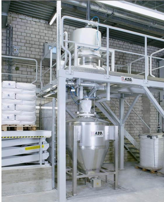
Unit for filling of DOSITAINER® with product out of sacks
