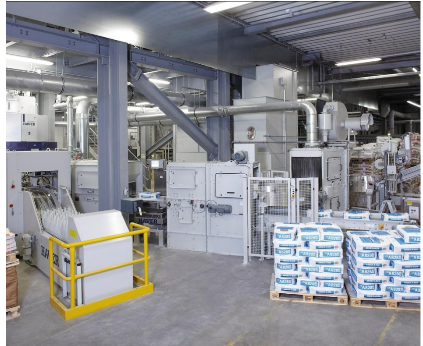
Packing of finished product in sacks
