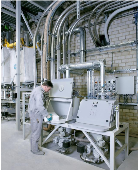
Feeding hopper with central aspiration
