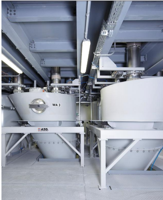
Hopper scales with 3-point weighing unit
