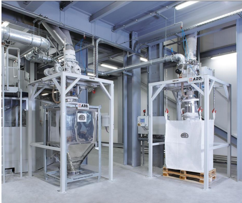
Container and big bag filling station
