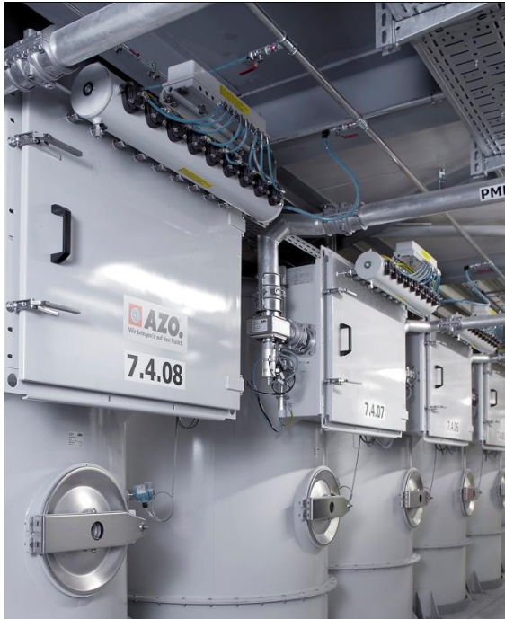
Buffer bins for temporary storage of products
