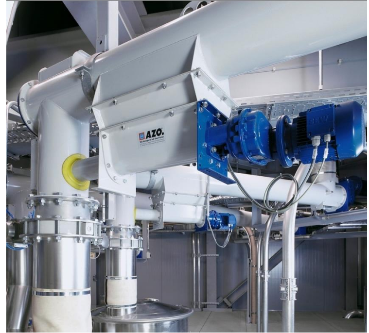
Dosing screw with fine dosing
