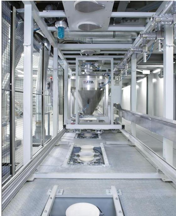
Container on travelling scale for collecting and weighing of the components
