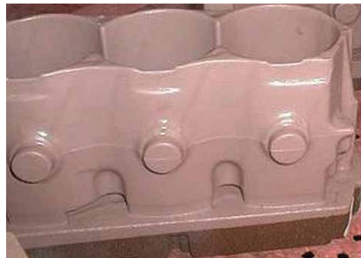
Figure 7: RHEOTEC XL coated water-jacket core and resulting defect free internal finish
