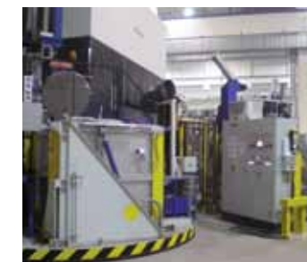
Flexible melt provision through two holding crucible furnaces on a rotary table
