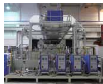
Die cooling with Robamat temperature control units
