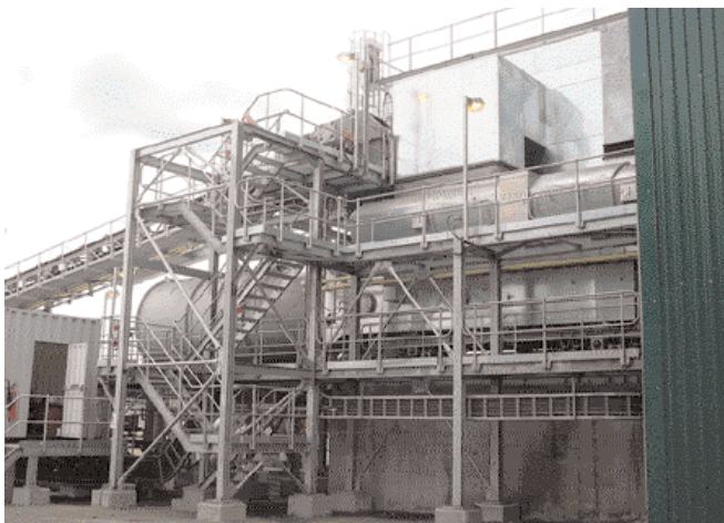
The dry plant showing part of the sand dryer, fluidised bed and dust extractor
