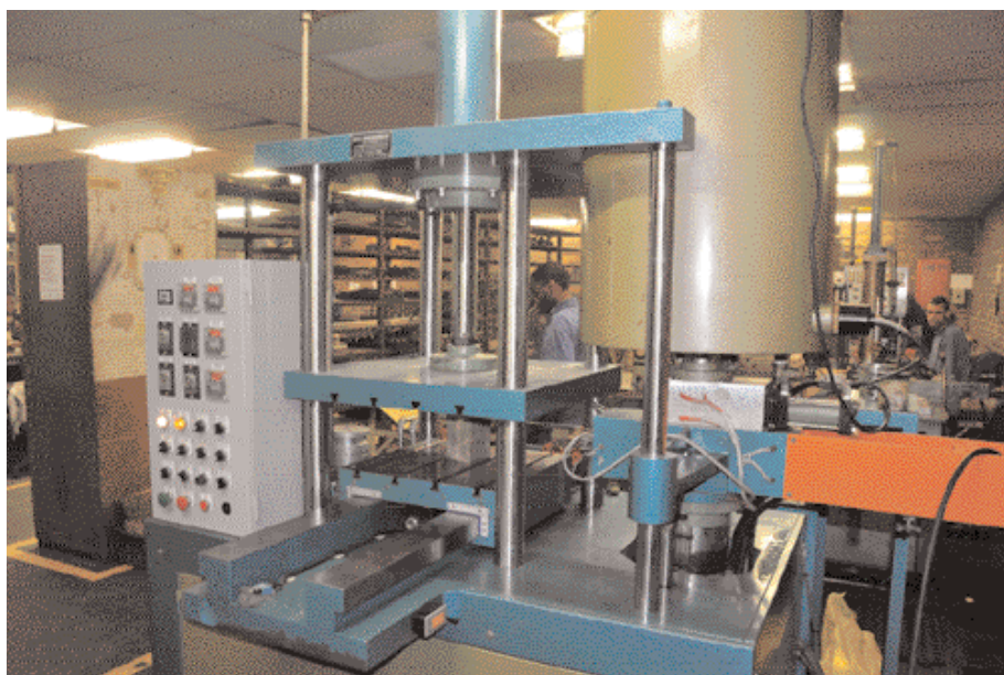
The second new Gifo double head wax injection press that can handle dies up to 500 mm wide
