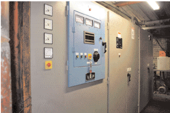
The new 1000 kW Inductotherm VIP® Induction Power Supply unit
