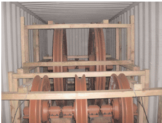
KEW Foundries is the sheave wheel supplier for the largest joint sector hydroelectric project in India. The diameters of the 43 sheave wheels supplied for this project range from 960mm to 2 555mm
