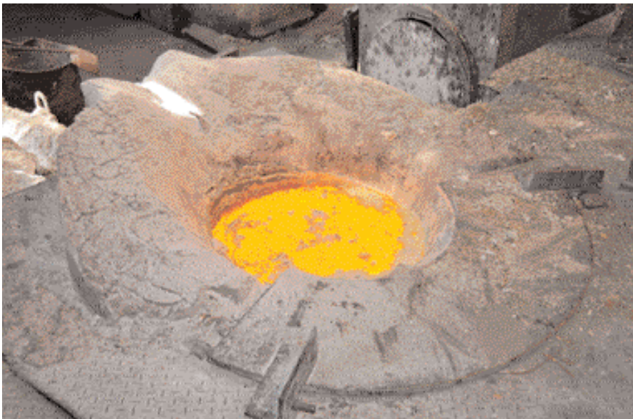
The new power supply unit has been installed in the non ferrous foundry division of Copalcor and is being used to melt commercial brass and copper alloys in an existing three ton furnace
