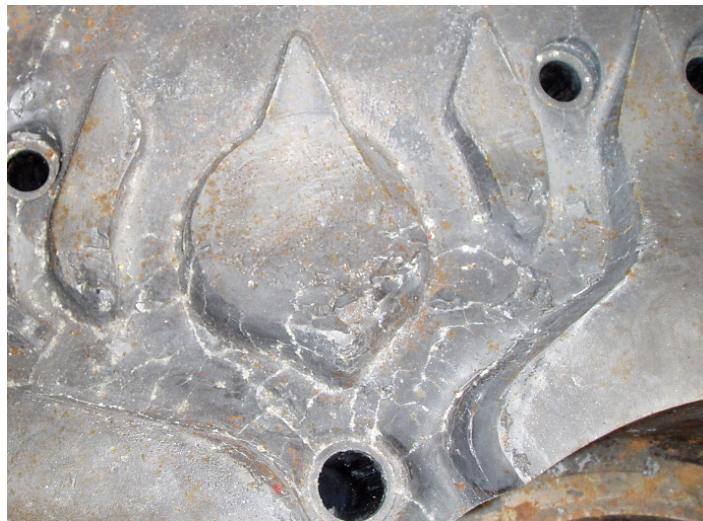
Fig. 1: Thermal-fatigue crack network on a die-casting die surface after approx. 110,000 cycles.
