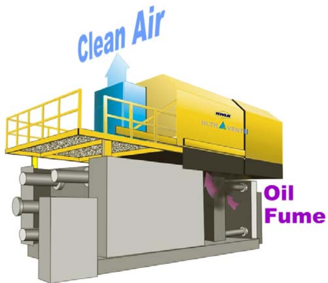
Scheme of a KMA ULTRAVENT filter system above a DCM
