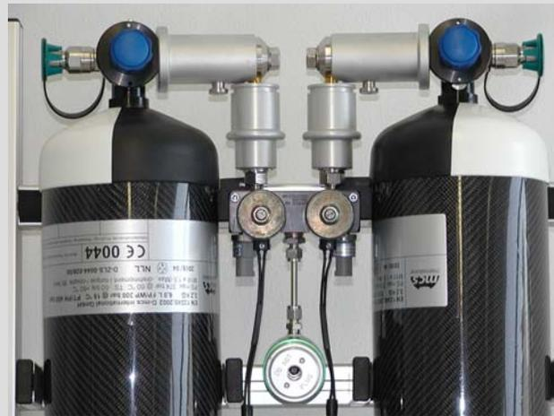
To facilitate the use of CLEVER in these regions, the vehicle is equipped with two gas cylinders that can be externally refilled after removal from CLEVER. Therefore, it is possible to exchange the cylinders e.g. at normal gas stations or supermarkets. However, the central refilling of both cylinders at public refuelling stations is also possible.
