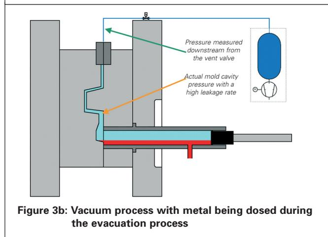
**Figure 3b: Vacuum process with metal being dosed during the evacuation process**
