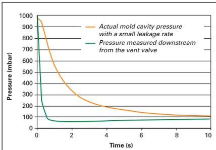
**Figure 5: Measured and actual pressures with a relatively tight mold**
