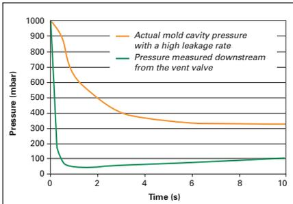
**Figure 4: Measured and actual pressures with a relatively leaky mold**
