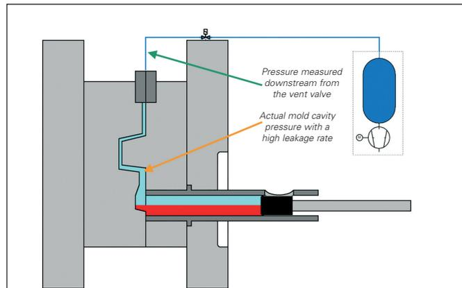
**Figure 3a: Standard vacuum process for die casting**
