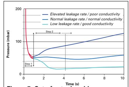
**Figure 7: Set of actual mold pressure curves with the two-step process**
