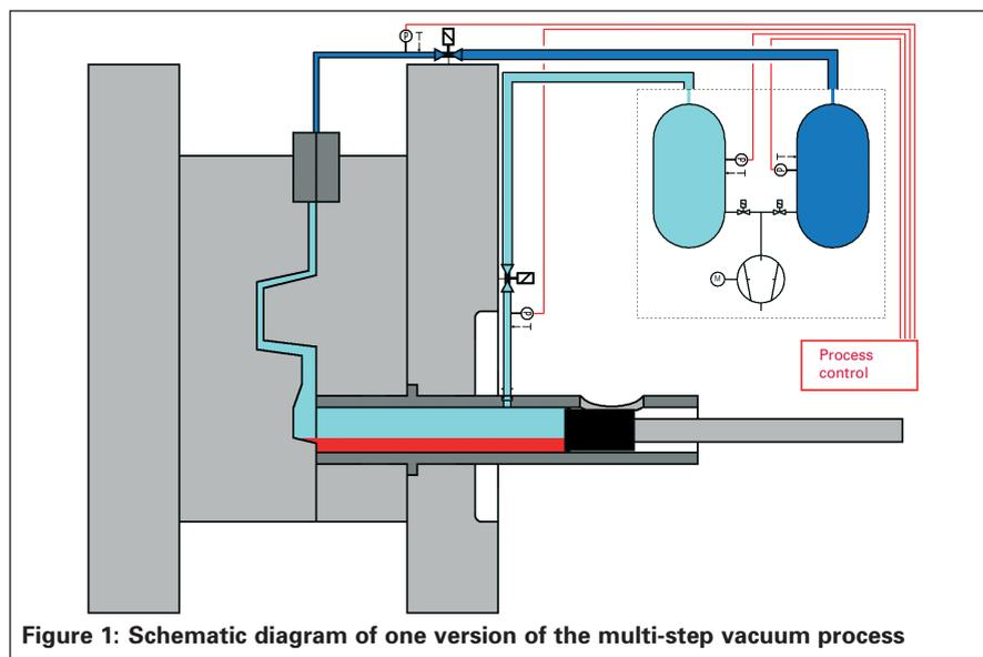
Figure 1: Schematic diagram of one version of the multi-step vacuum process
