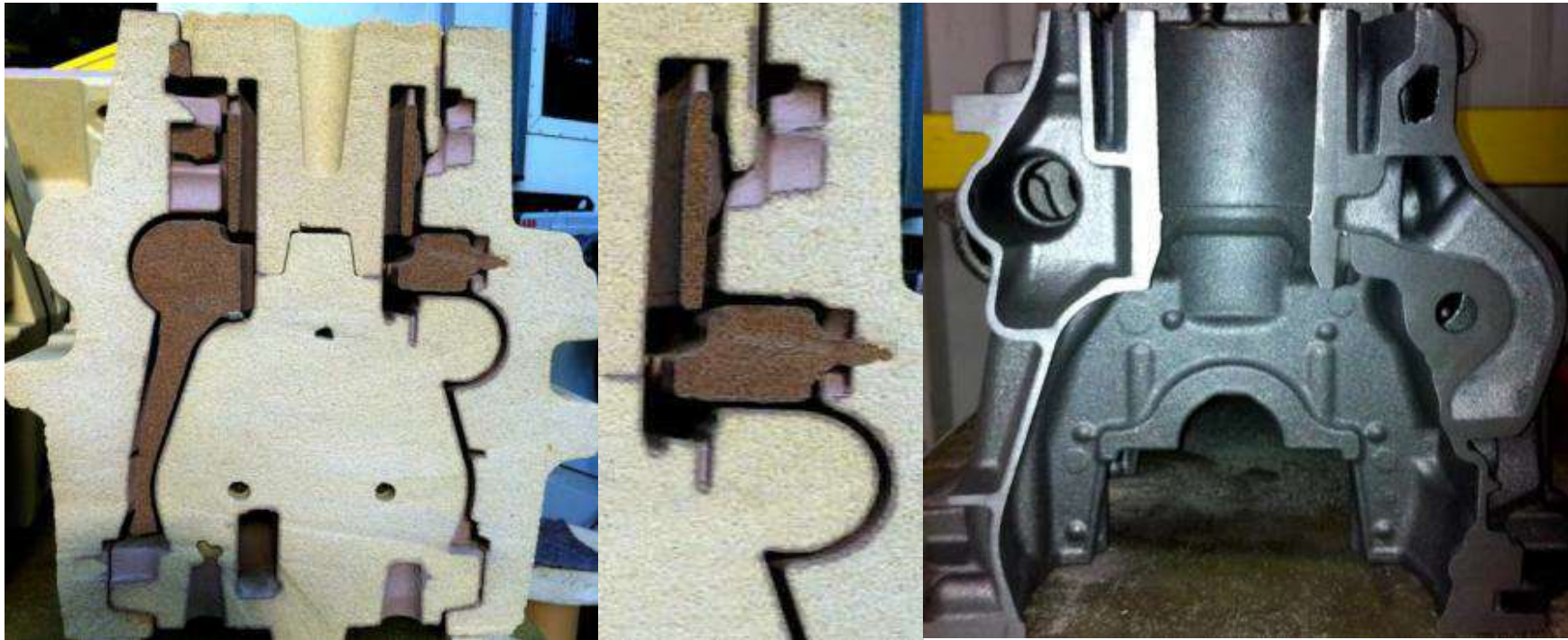
Section through a core package in casting position by cutout over a range of core and a section of the corresponding cylinder block
