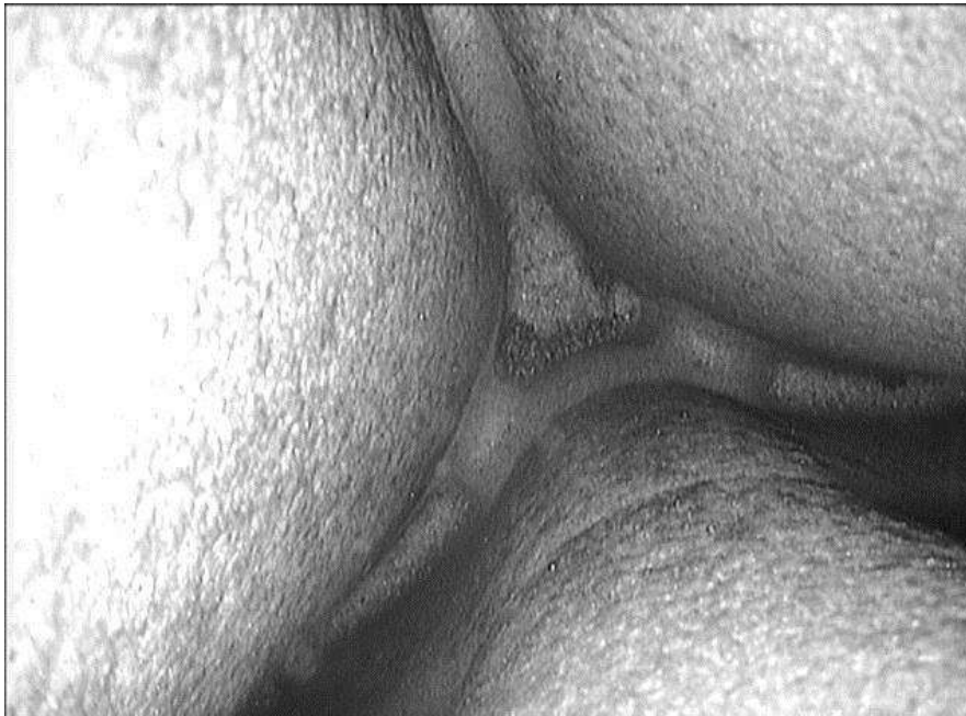
Extensive sticking of the refractory coating on the casting surface
