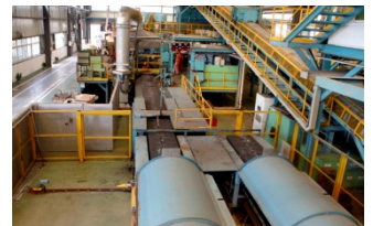
DISA 231 – vertical line with shuttle system
