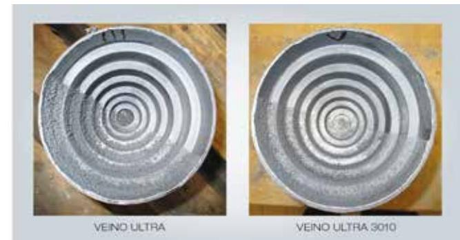
Figure 3: Comparison between VEINO ULTRATM and VEINO ULTRATM 3010 additive, half-coated
