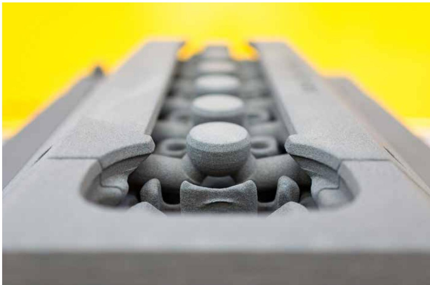
*Christenguss AG already generates complex sand casting molds in the 3D printing process.*
