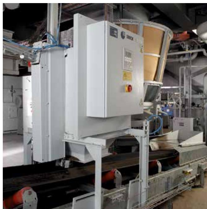
QualiMaster AT12 moulding sand online inspection device (Photo: Eirich)
