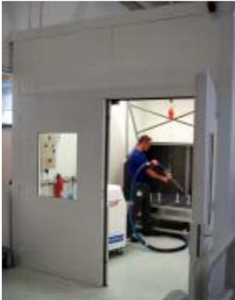
ASCO has delivered a complete dry ice cleaning solution including noise control booth to DaimlerChrysler. The noise control booth is in the motor assembly factory in Bad Cannstatt, where silicon residues are removed from motor parts by a dry ice blasting unit type ASCOJET 2001RS.
