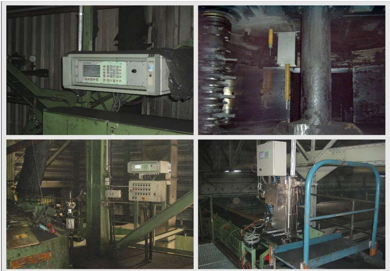
Fig. 1 Measuring and control system components installed in the sand preparation shop: moisture measuring and control system Micomp UNI type G-MC mounted on the cooler (above left), self-cleaning electrode and temperature sensor in the mixer (above right), moisture measuring and control system MICOMP UNI type G-CH mounted on the mixer (below left), sand-testing system VEDIMAT (below right).
