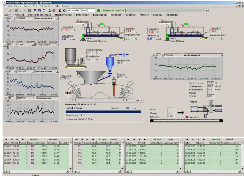
Fig. 2 MiPro overview with individually displayed plant components (mixer with primary moisture measurement, two coolers, one mechanical sand-testing system)
