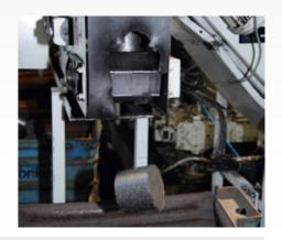
Briquetting system: RUF 30/3700/100 (adapted model)
